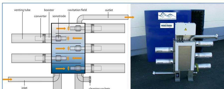
**Figure 2.** Ultrawaves ultrasound reactor. Standard unit of 5 kW.
