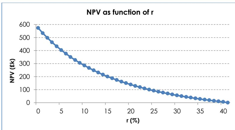
**Figure 6:** NPV as function of  $r$  for the 5 kW unit performing in WwTW-AD.
