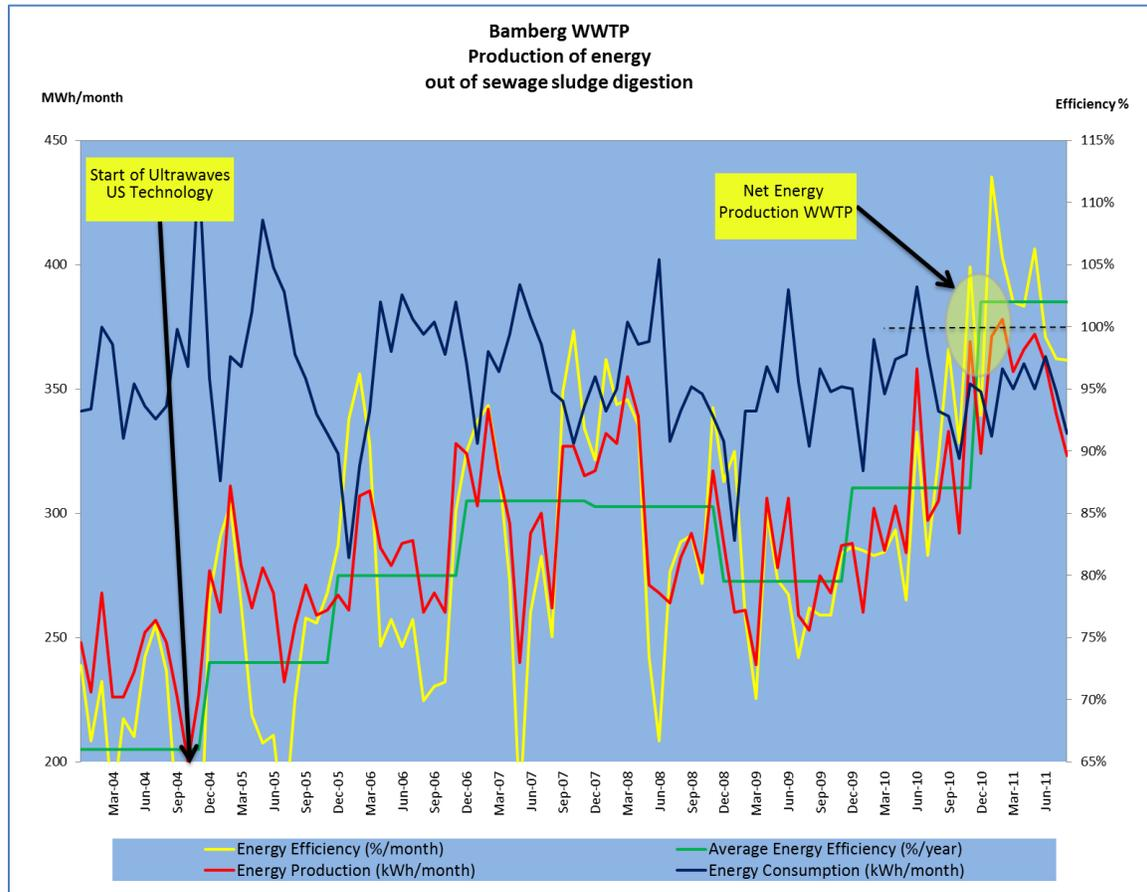
**Figure 1:** Ultrawaves performance at Bamberg WWTP since 2004.
