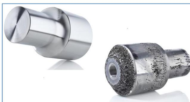
**Figure 5:** New sonotrode and after 1.5 to 2 years running.
