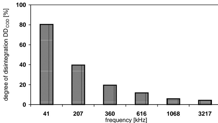
**Figure 3.** Effect of ultrasonic frequency on the degree of cell disintegration (TSS: 20 g/L, ultrasound intensity: 1.8 W/cm<sup>2</sup>, sonication time: 4 h).
