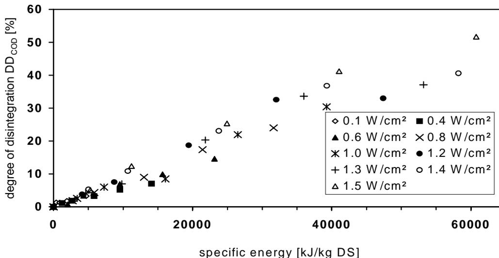
**Figure 5.** Effect of intensity and energy dose at 41 kHz on the degree of disintegration of sewage sludge bio-solids (lab reactor URS 1000, L-3 Communications ELAC Nautic, Kiel, Germany; sonication time: max. 2 h; bio-solids as dry solids (DS) weight concentration : 25.9 g/kg).
